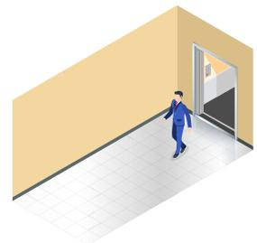
Present a card or a QR Code or verify the identify by facial recognition at the entrance control point. The screen will display the assigned elevator number and the destination floor.
