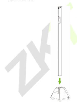
Insert the pole into the hexagonal slot of the base.
