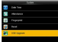
Insert the U disk with upgrade file into the device's USB port, and in the initial interface, press [M/OK] >
