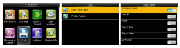
In the initial interface, press [M/OK] > Print > Data Field Setup > press [M/OK] to turn on / off the fields needing to be printed.
