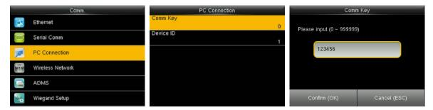
In the initial interface, press [M/OK] > Comm. > PC Connection > Comm Key to enter the Comm Key setting interface.
