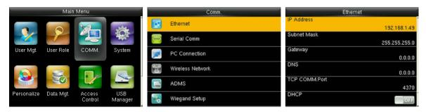
In the initial interface, press [M/OK] > Comm. > Ethernet to enter the Ethernet setting interface.
