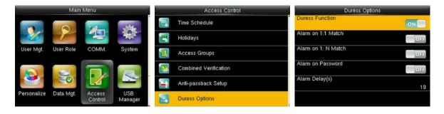
Setting Duress Key: In the initial interface, press [M/OK] > Personalize > Shortcut Key Mappings > select the [M/OK] key > press [M/OK] > Function > select the "Duress Key" option. (The Duress Key menu will be displayed after the Duress Function is turned on.)
