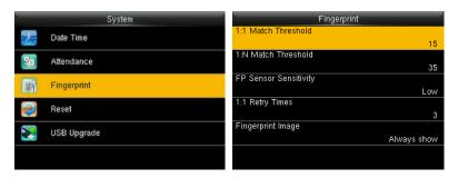
In the initial interface, press [M/OK] > System > Fingerprint to enter the Fingerprint setting interface.
