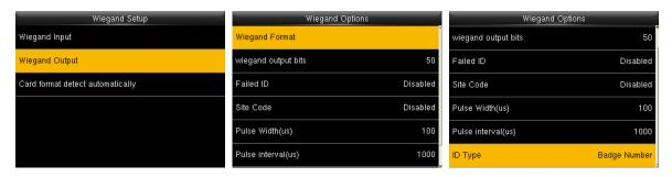
**Wiegand Format:** User can choose among the following built-in Wiegand formats: Wiegand 26, Wiegand 26a, Wiegand 34a, Wiegand 36a, Wiegand 36a, Wiegand 37, Wiegand 37a and Wiegand 50. Multiple selections are available, but the actual Wiegand format will depend on the option in **[Wiegand output bits]**.
