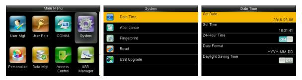
In the initial interface, press **[M/OK]** > **System** > **Date Time** to enter the date/time setting interface. It includes setting date, time, 24-hour clock, date format and daylight saving time.
