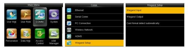
In the initial interface, press [M/OK] > Comm. > Wiegand Setup to enter the Wiegand Setup setting interface.
