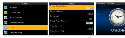
In the initial interface, press [M/OK] > Comm. > ADMS to enter the ADMS server setting interface. When the Webserver is connected successfully, the main interface will display the logo.
