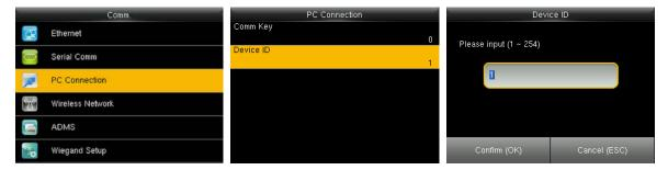
In the initial interface, press [M/OK] > Comm. > PC Connection > Device ID to enter the Device ID setting interface.
