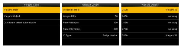
**Wiegand Format:** User can choose among the following built-in Wiegand formats: Wiegand 26, Wiegand 26a, Wiegand 34, Wiegand 34a, Wiegand 36a, Wiegand 37, Wiegand 37a and Wiegand 50.
