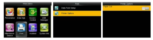
In the initial interface, press [M/OK] > Print > Printer Options > press [M/OK] to turn on / off the Paper Cut function.
