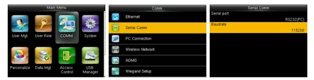
In the initial interface, press **[M/OK]** > **Comm.** > **Serial Comm** > **Baudrate** to enter the **Baudrate** setting interface.
